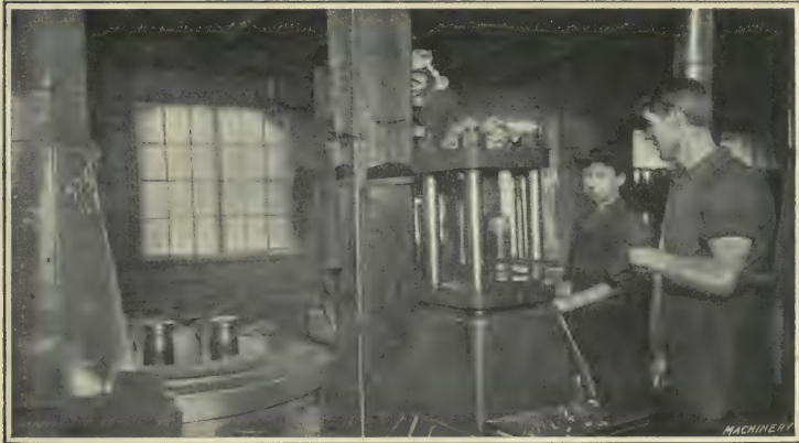
Fig. 15. Closing in Nose of Shrapnel Shell in Hydraulic Press
